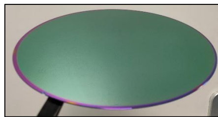
Figure 2. 200mm GaN grown by MBE
