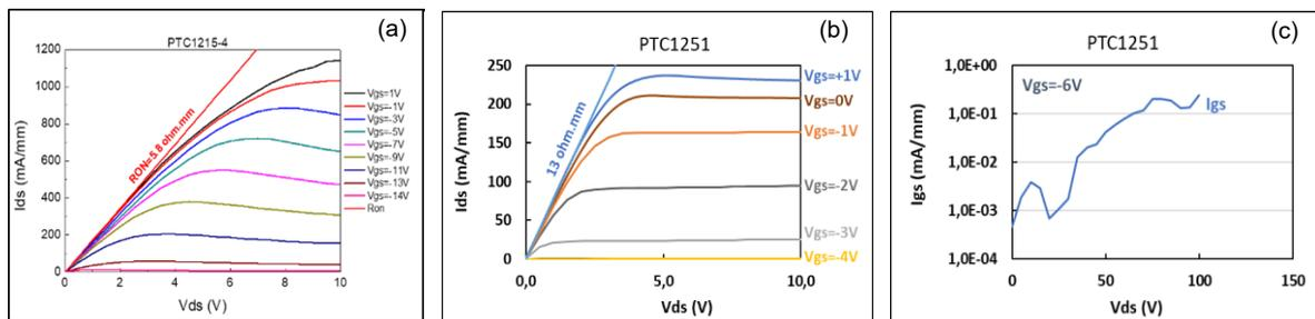
Fig. 4: DC output characteristics  $I_{ds}(V_{ds}, V_{gs})$  of 2  $\mu\text{m}$  gate transistors with 9  $\mu\text{m}$  source-drain spacing fabricated on the ScAlN/GaN HEMT grown on Silicon with (a) a 25 nm barrier and (b) a 10 nm barrier. (c) Gate leakage of the 10 nm barrier HEMT in 3-terminal off-state configuration.
