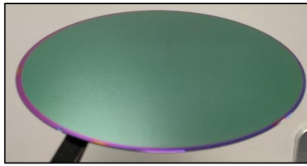
Figure 2. 200mm GaN grown by MBE
