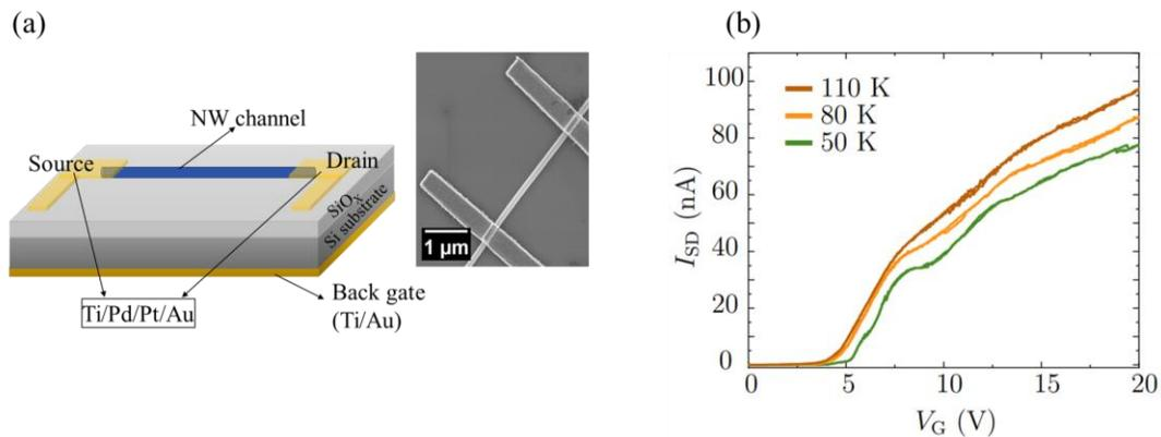
Fig. 3: (a) Schematic (left) and SEM image (right) of a NW field effect transistor (FET) with metallization profile used for InAs-AISb core-shell NWs with GaSb cap; (b) temperature-dependent transfer characteristic of the NW-FET at varying temperatures of 50 K, 80 K and 100 K.
