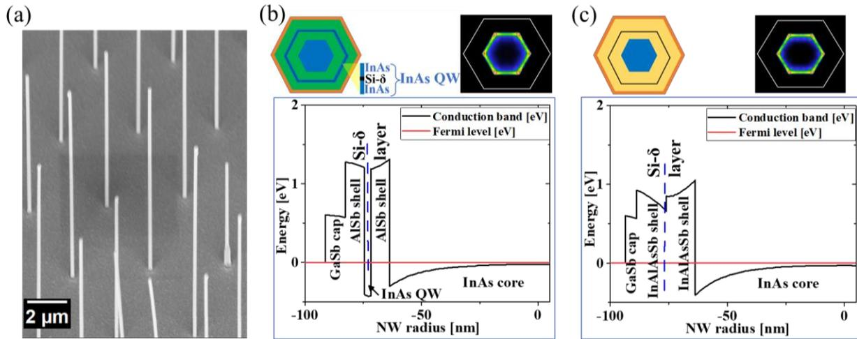
Fig. 1: MBE grown core-shell NWs and simulation data for different modulation doped structures; (a) InAs-AISb core-shell NWs obtained by selective area epitaxy on prepatterned SiO<sub>2</sub>/Si (111) substrate; (b,c) Schematic cross-section, band profiles, and corresponding electron density maps of (b) InAs-AISb core-shell NW with InAs QW hosting a Si- $\delta$  layer, and (c) InAs-InAlAsSb core-shell NW with Si- $\delta$  doping layer at the center of the shell.
