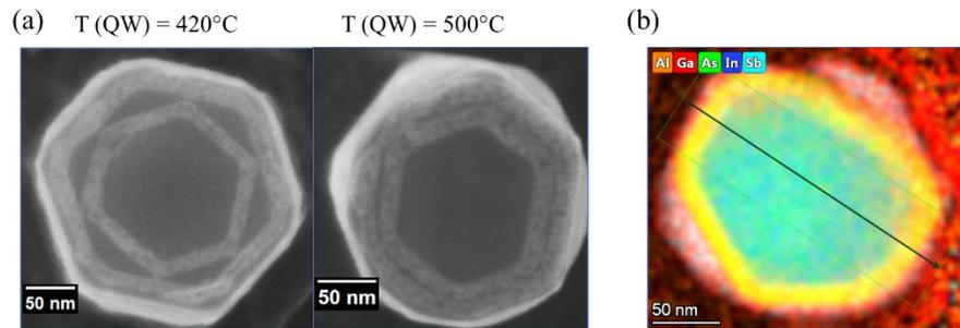
Fig. 2: (a) Helium ion microscopy (HIM) images of InAs-AISb core-shell NWs with InAs QW embedded in the shell, for QW growth temperature of 420 °C (left, asymmetric growth) and 500 °C (right, symmetric growth); (b) STEM-EDX compositional map of the elemental distribution within an InAs-InAlAsSb core-shell NW.
